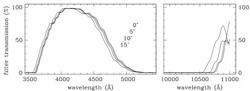
Fig. 3: Transmission profiles (measured on September 2011) under various angles of incidence of the light beam (expressed as deviations from 90° normal incidence), for an old Astrodon Johnson B filter in use since December 2009 at ANS Collaboration telescope R122.
