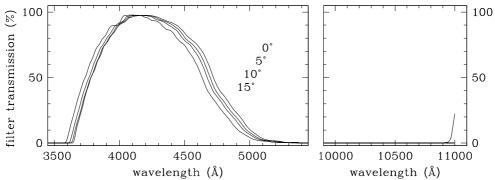
Fig. 4: Similar to Fig. 3 for a test article of the new Astrodon Johnson B filter (red-leak suppressed) measured on April 2012.
